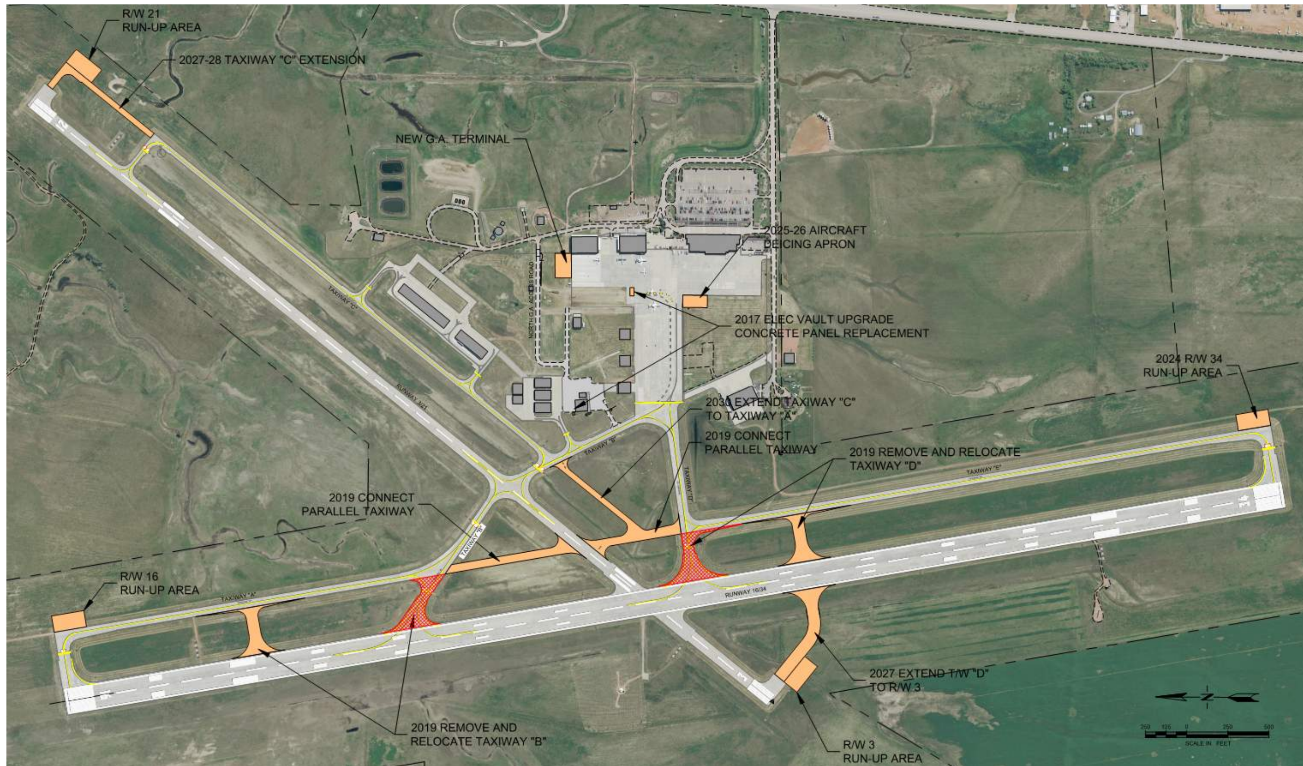
Figure 4-3. Potential Taxiway Extensions and Removals
